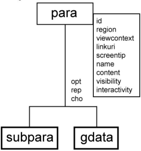
Figure 2d. WebCGM File Structure - PARA
